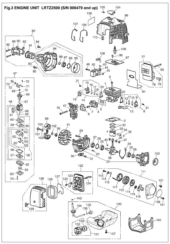
Fig.3 ENGINE UNIT LRTZ2500 (S/N 000479 and up)
